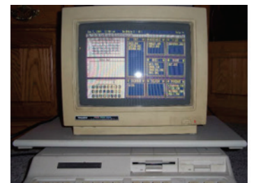
Tandy 1000 HX circa 1987. Personal DeskMate GUI. Note high class dual floppy drives. 640 k RAM. No hard drive.
